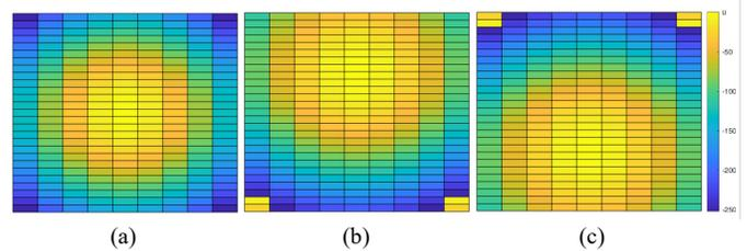
Fig. 5. The required reflection phase when scan angle is (a) $0^\circ$ , (b) $15^\circ$  and (c) $-15^\circ$ .
