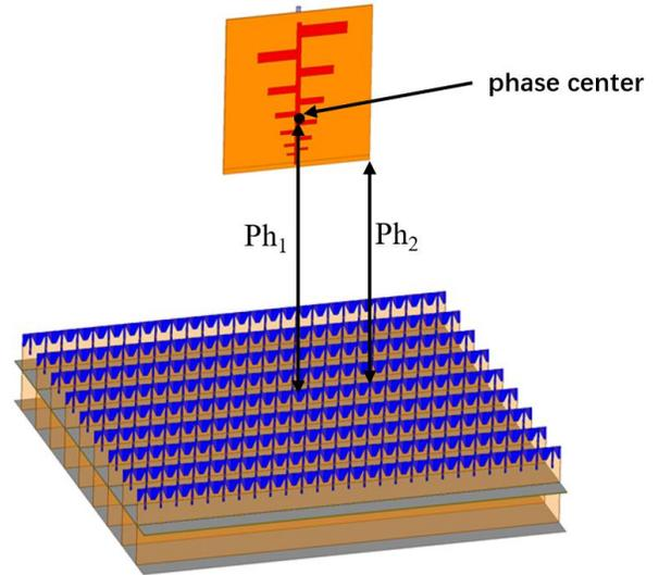
Fig. 4. Configuration of the reflectarray.
