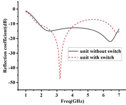
Fig. 2. The reflection coefficient of the element.
