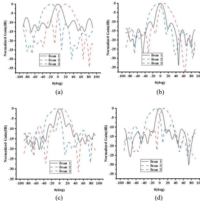
Fig. 7. Simulated radiation patterns at (a) 3.5 GHz, (b) 4 GHz, (c) 4.5 GHz and (d) 5 GHz.
