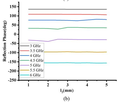
Fig. 3. The reflection phase of the element when the switch is (a)ON, (b)OFF
