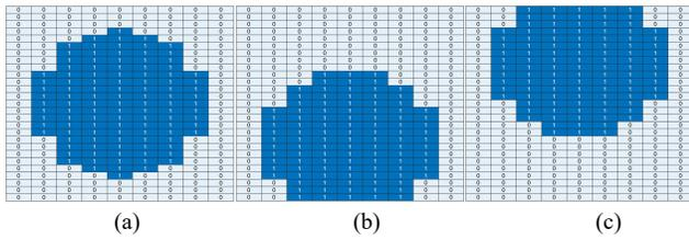
Fig. 6. The status distribution when scan angle is (a)  $0^\circ$ , (b)  $15^\circ$  and (c)  $-15^\circ$ .
