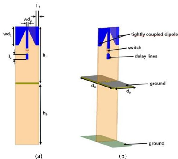
Fig. 1. The configuration of the proposed unit (a) front view, (b) side view.
