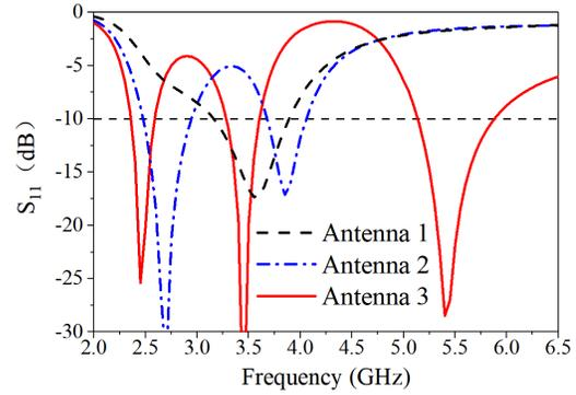
Fig. 3. Simulated  $|S_{11}|$  of various antennas involved in Fig. 2
