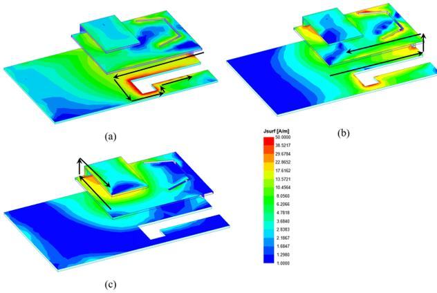
Fig. 5. Simulated surface current distributions of the proposed antenna at (a) 2.5, (b) 3.5, and (c) 5.5 GHz.
