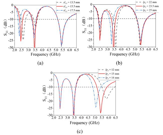
Fig. 6. Simulated  $|S_{11}|$  of the proposed antenna for various (a)  $sl_{11}$  (b)  $lp_1$  (c)  $lp_2$
