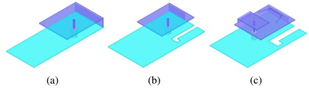
Fig. 2. Design evolution of the proposed antenna (a) Antenna 1 (b)Antenna 2 (c)Antenna 3
