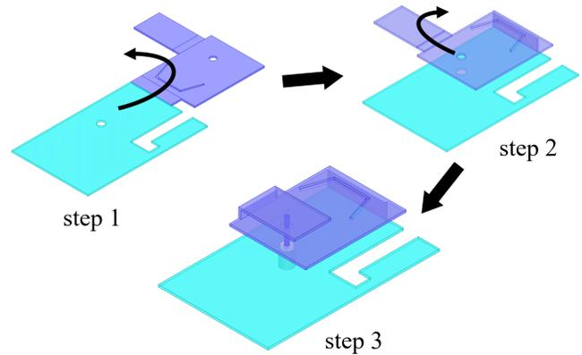
Fig. 4. Manufacturing steps of the proposed antenna
