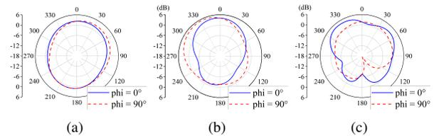
Fig. 7. Radiation patterns for the proposed antenna at (a) 2.5, (b) 3.5, and (c) 5.5 GHz.
