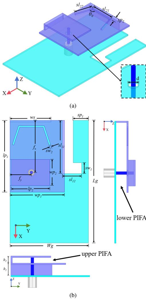
Fig. 1. Geometry of the proposed antenna (a) Perspective view. (b) Composite views
