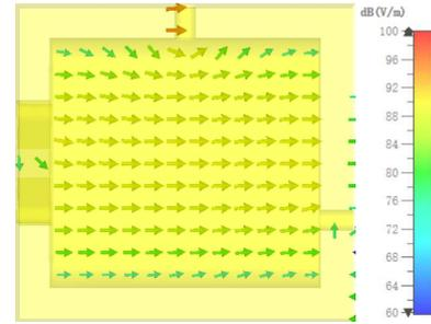
Fig. 7. Cavity internal electric field at 28.1 GHz.
