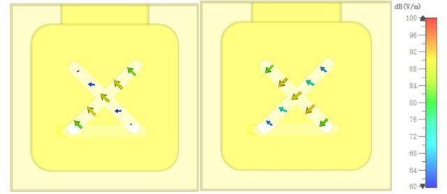
Fig. 6. Cavity slot electric field at 27.24 GHz. (a)  $t=0$ . (b)  $t=T/4$ .
