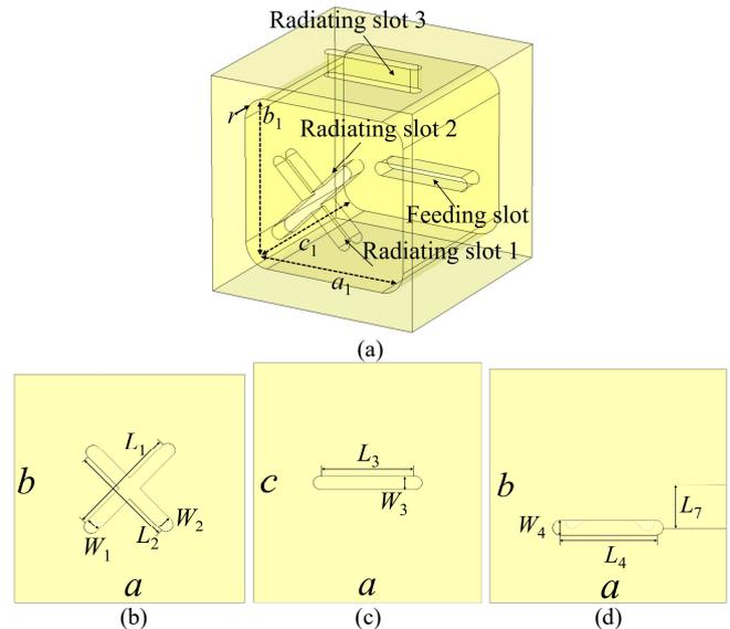
Fig. 2. Antenna structure. (a) 3-D view. (b) Front view. (c) Top view. (d) Rear view. Physical dimensions (units: mm):  $L_1 = 4.4$ ,  $L_2 = 4.2$ ,  $L_3 = 3.9$ ,  $L_4 = 3.7$ ,  $a = 9.4$ ,  $a_1 = 7.4$ ,  $b = 9.4$ ,  $b_1 = 7.4$ ,  $c = 9.9$ ,  $c_1 = 7.9$ ,  $W_1 = 0.6$ ,  $W_2 = 0.6$ ,  $W_3 = 0.6$ ,  $W_4 = 0.6$ .
