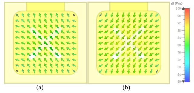
Fig. 5. Cavity internal electric field at 27.24 GHz. (a)  $t=0$ . (b)  $t=T/4$ .
