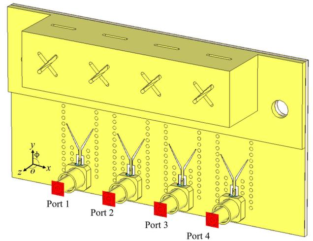
Fig. 10. Simulated antenna array structure.
