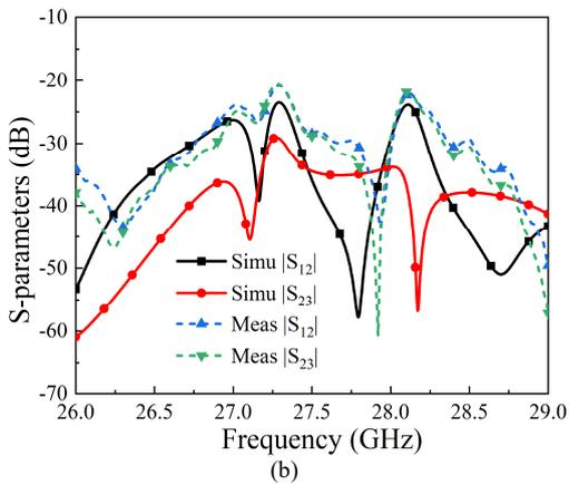
Fig. 12. Simulated and measured S-parameters of the antenna array.
