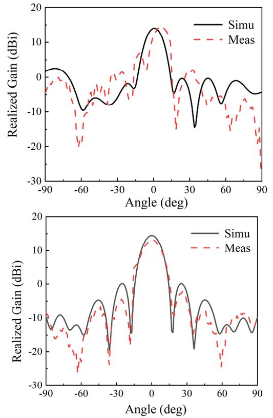
Fig. 13. Simulated and measured antenna array radiation patterns. (a) 27.24 GHz. (b) 28.1 GHz.
