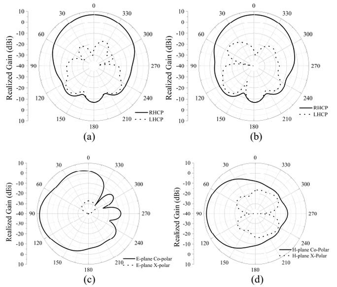
Fig. 9. Simulated antenna radiation patterns. (a) xoz plane 27.24 GHz. (b) yoz plane 27.24 GHz. (c) yoz plane 28.1 GHz. (d) xoy plane 28.1 GHz.
