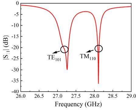
Fig. 3. Simulated parameters of  $|S_{11}|$ .
