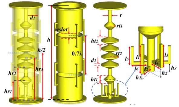
Fig. 5. Structural diagram of the filtering antenna. (a) Three-dimensional view. (b) External structural diagram. (c) Internal structural diagram.
