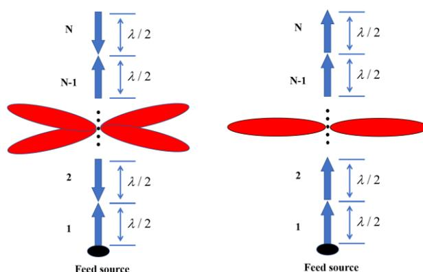
Fig. 1. Schematic diagram of a series-fed antenna array: (a) before phase correction, (b) after phase correction.
