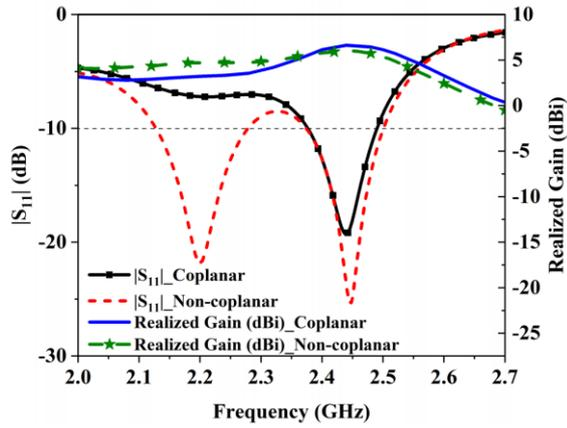
Fig. 3. Simulated  $|S_{11}|$  and realized gain of coplanar structure antenna and non-coplanar structure antenna.
