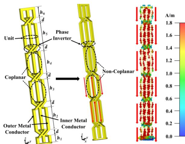
Fig. 2. (a) Coplanar structure antenna. (b) Non-coplanar structure antenna. (c) Simulated current distributions of the non-coplanar structure antenna. (Physical dimensions, all units are in mm:  $h_1 = 17$ ,  $h_2 = 36$ ,  $h_3 = 34$ ,  $h_4 = 40$ ,  $h_5 = 34$ ,  $h_6 = 24$ ,  $d = 9$ ).
