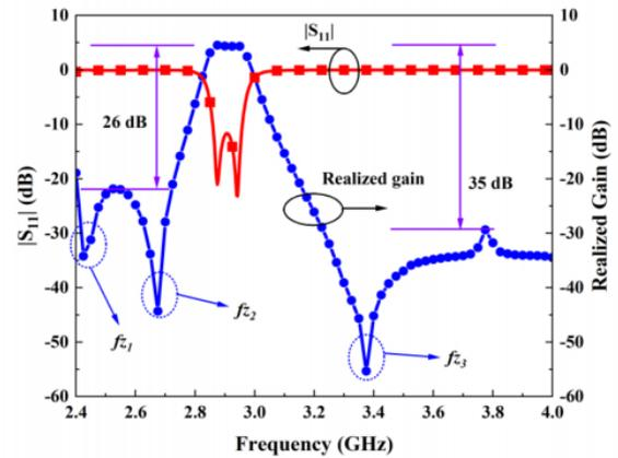
Fig. 6. Simulation S parameter and gain curve of the filtering antenna.
