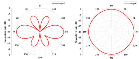
Fig. 7. (a) E-plane radiation patterns of the filtering antenna. (b) H-plane radiation patterns of the filtering antenna.
