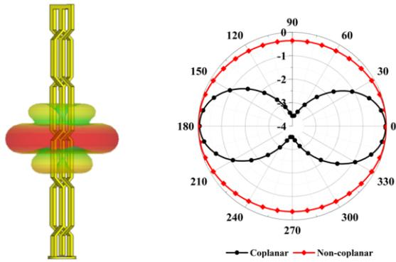
Fig. 4. (a) Simulated 3-D radiation pattern of non-coplanar structure antenna. (b) H-plane radiation patterns of coplanar and non-coplanar structure antenna.
